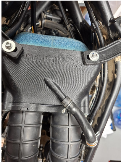
NoBrand Performance Airbox positioned on the motorcycle. Reuse the OEM mounting bolts and spacers at the frame mounting points.
