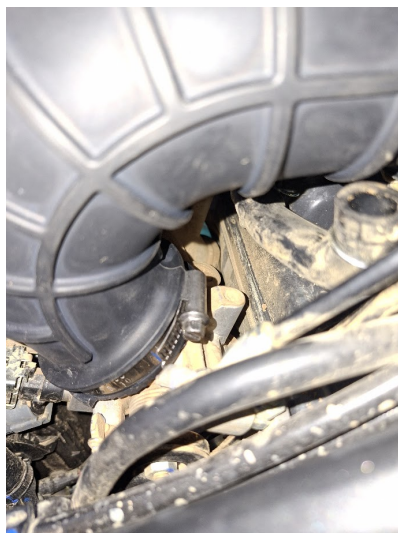
Performance-airbox installation reference: intake/throttle-body area after positioning the new airbox. Confirm correct seating and clearance.
